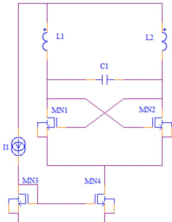
The Fig. 2 topology solves the undefined current problem, but adds noise from the current source. The current source noise is minimised when there is a 1:1 ratio of current to the input of the mirror and the mirror output, however this doubles the total supply current.
