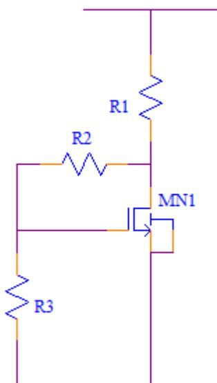
Fig. 3 illustrates a standard “ $V_{be}$  multiplier”. MN1 is typically biased so that it runs with low  $V_{gst}$  and allows for its drain voltage to be multiplied up from round about its  $V_{th}$ . The drain current is thus set fairly accurately at the supply voltage minus  $V_d$  divided by  $R$ . Typically around 20% in operating current might be achieved.
