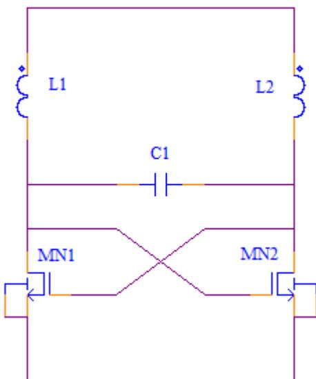
Fig. 1 is the standard differential oscillator topology. The issue with this circuit is that there is no defined operating current. It flaps in the wind based on the supply voltage and the gate threshold voltage. Quite possible a 10:1 variation in current, so not good news for a low power design.
