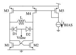
Figure 5: Oscillator with on-chip inductor
